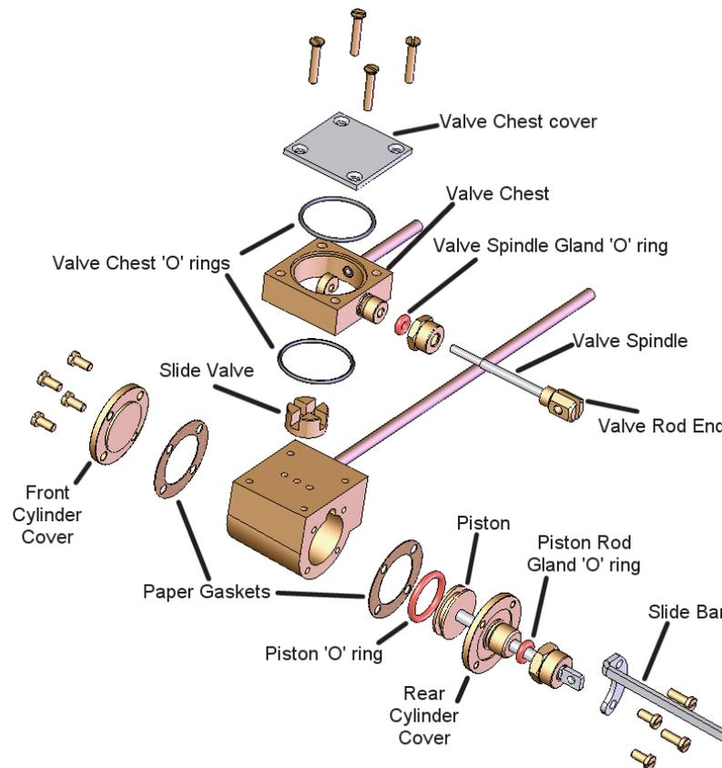
Round slide valve cylinder assembly. First introduced in 1999 on the 'basic series' locomotives but gradually phased in on 'classic series' models from 2002. There are several variations of this, some with sloping or smaller 3/4" square valve chests, but all are essentially of similar construction.
