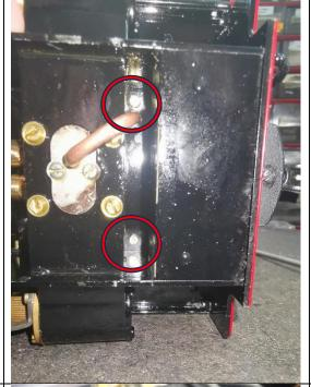
From underneath remove the other two screws holding the smokebox to the chassis.
