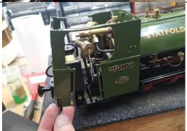
This should release the rear of the cab with the rear buffer beam.
