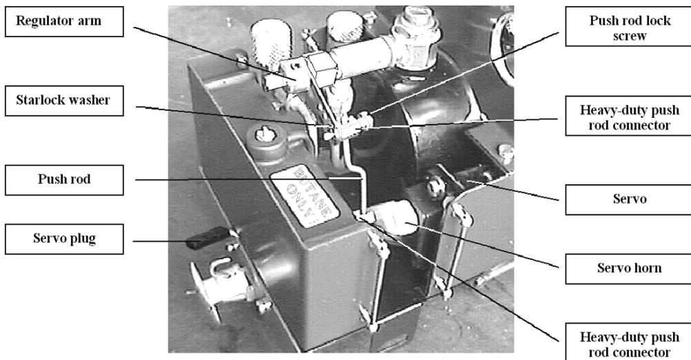
A replacement R/C type regulator is supplied with this kit. Although externally it looks the same as the manual type fitted to the loco, internally it is quite different. It is designed to operate with a servo where a small amount of movement must give full control from closed to fully open. It also relies on an internal 'O' ring to ensure that it closes fully with the minimum of force.
