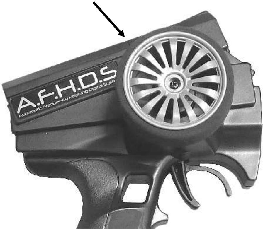
If continual running is desired, set the loco to the required speed and then switch off the power to the transmitter. The model will then continue to run at that speed. To re-gain control, switch the transmitter power back on again.
