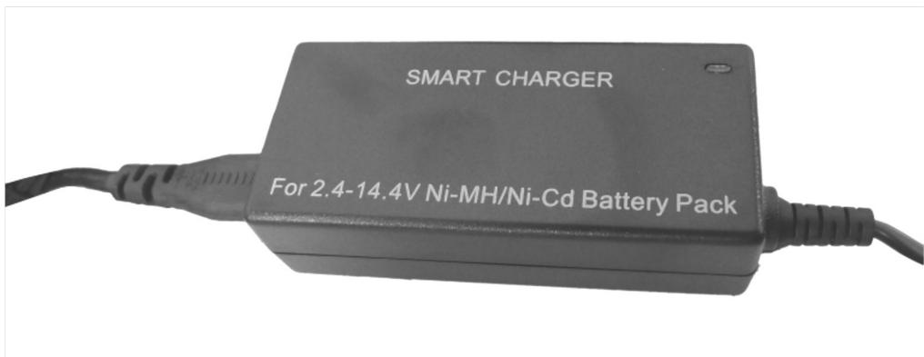
It will initially take approximately 5 hours for the batteries to fully charge. The time taken for subsequent full charges may be less. When the batteries are fully charged, the LED will change to green. The charging jack should now be removed from the locomotive and the charger unplugged from the mains.
