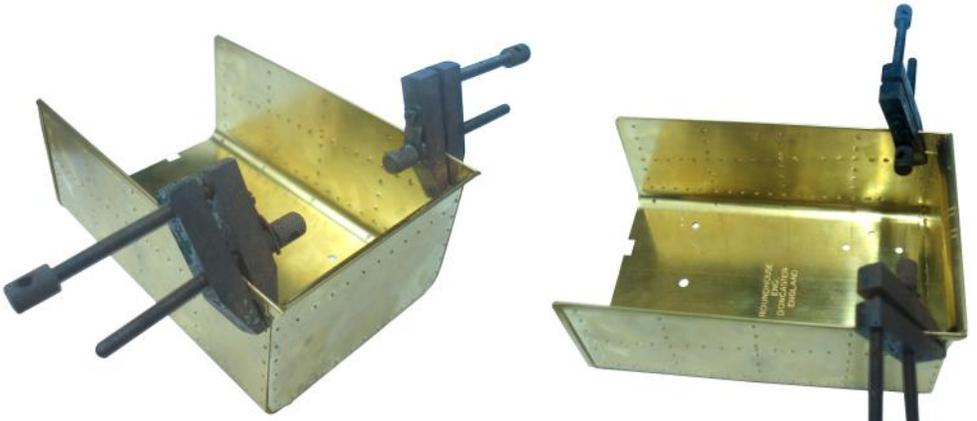
The tender front can now be soldered. Clamp the front into the tender body. Use the first vertical line of rivets on the tender to line up the front plate and ensure that the bottom flange is flush with the tender floor.
