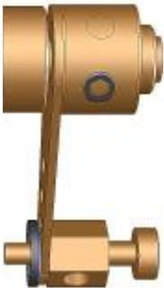
Gently turn the regulator arm clockwise with your fingers to close it, but do not force it. When closed, the regulator arm should be roughly parallel to the servo horn. If not, use the Allen key to loosen the grub screw and move the regulator arm to the correct position.
