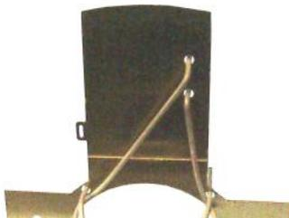
Cab front panel showing where the pipework fits.
