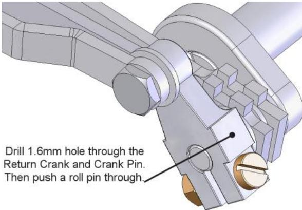
Drill 1.6mm hole through the Return Crank and Crank Pin. Then push a roll pin through.
