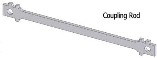
Place a 5BA steel washer over one of the rear crank pins and then push a coupling rod on after it, checking that the two lugs are pointing to the top. Connect the front end of the coupling rod to its outside crank using a short crank pin with another 5BA steel washer between the rod and the crank. Repeat for the opposite side.
