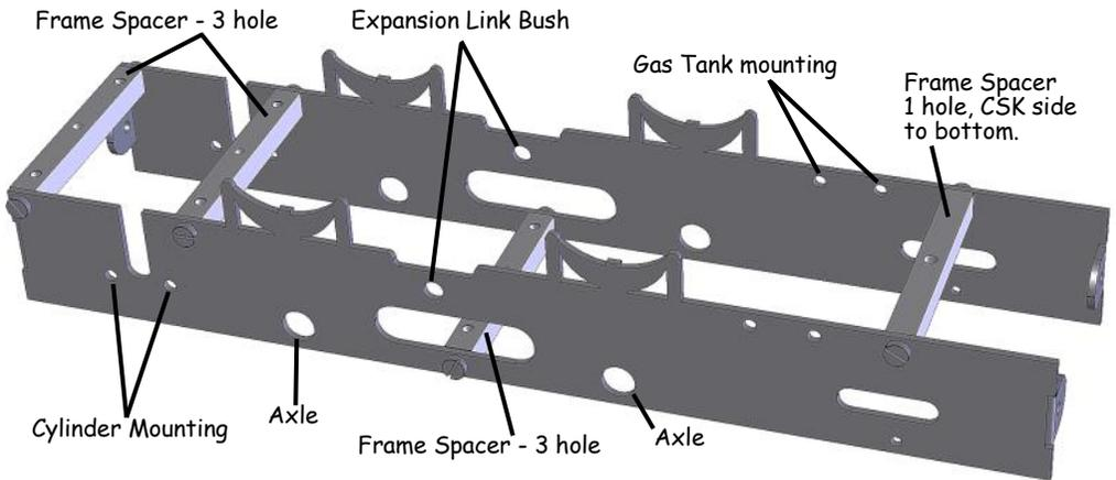
Refer to the diagram above and note the position of the four frame spacers. All the Frame Spacers should be positioned as shown, with the holes sitting vertically. The rear Frame Spacer has one untapped hole, with the countersunk (CSK) side to the bottom of the frame.
