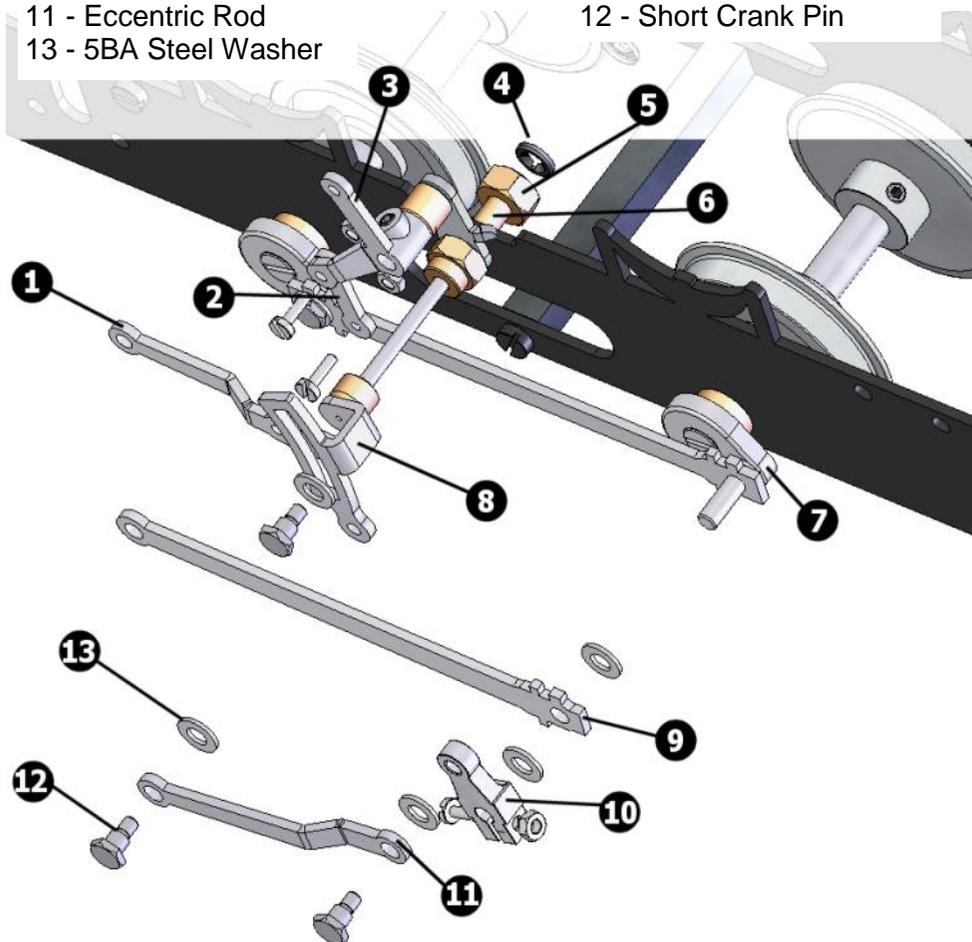
Refer to the diagram below and note that the return crank always leads the crank pin in forward rotation.
