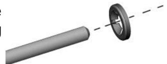
The eccentric rods can now be fitted to connect the return cranks and the expansion links. These rods are slightly tapered and the thicker end has a 'joggle'. They are attached by 6BA shouldered crank pins with a 5BA steel washer between. The thicker end goes
