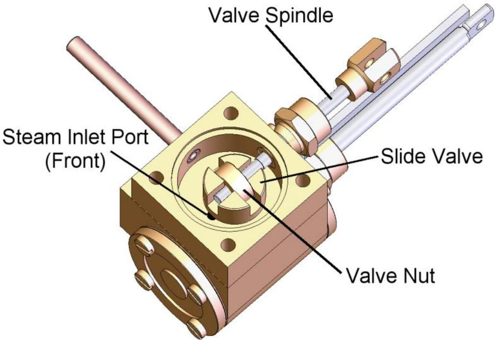
the crank pin on the drive axle is at dead centre. The front steam port should be cracking open at front dead centre and the rear steam port at rear dead centre.
