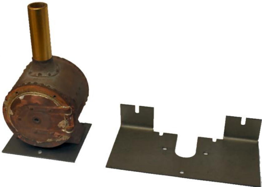
Smoke box footplates—Katie on the left and George on the right.
