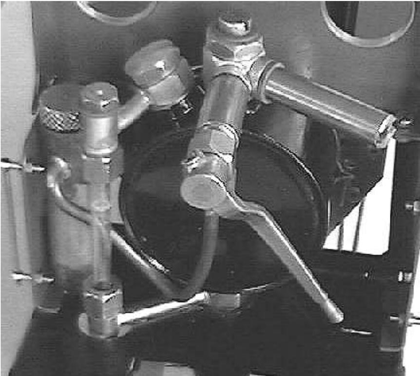
Fit the new turret to the top of the boiler with new copper sealing washers and tighten the top nut with the box spanner. Re-connect the steam pipe to the regulator.
