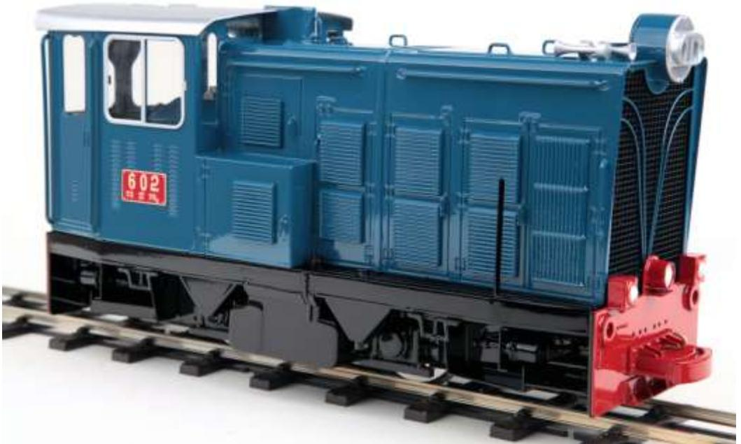
Built by Suri and Nayar (SAN) Engineering & Locomotive Company, Bangalore, this locomotive is currently operated by the Darjeeling Himalayan Railway. The loco is a 2-axle, air-braked unit, weighs in at around 17.5 tonnes and is powered by a Kirloskar-Cummins engine with 335 hp continuous output. The NDM-6 is the fourth in our series of battery powered diesel models.
