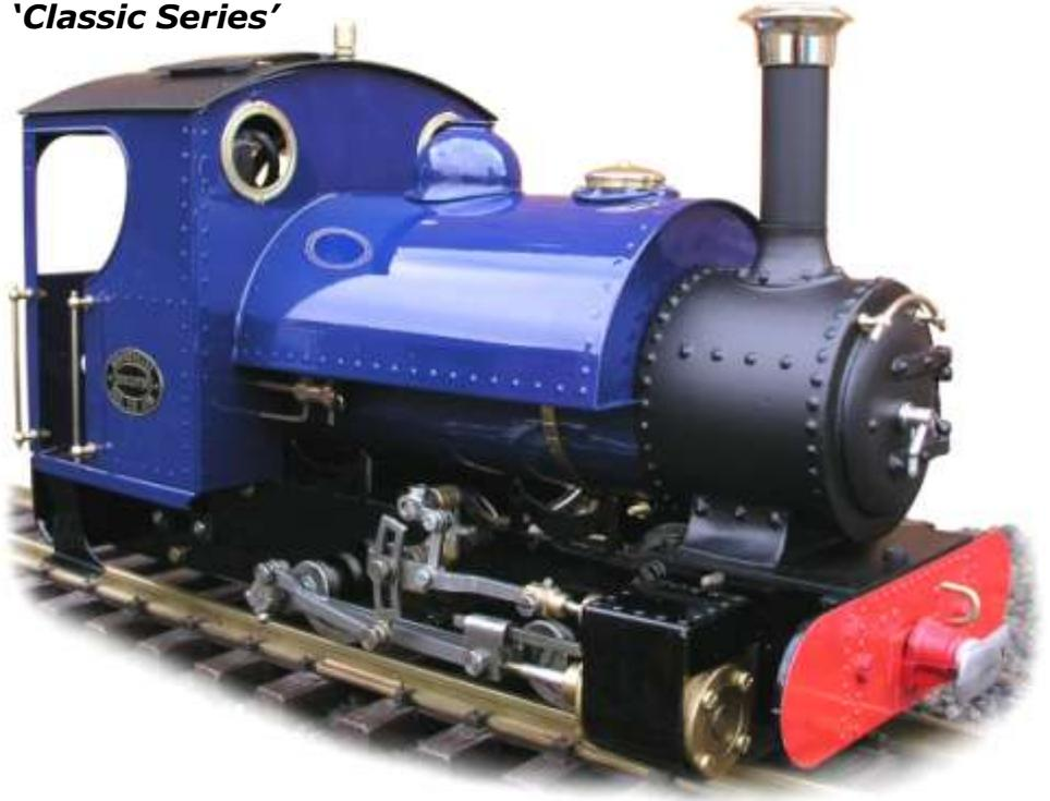
Katie is of typical narrow gauge saddle tank locomotive design. Though not a model of any particular engine, she draws inspiration and features from a number of famous builders like Hunslet, Bagnall and Pecket etc.
