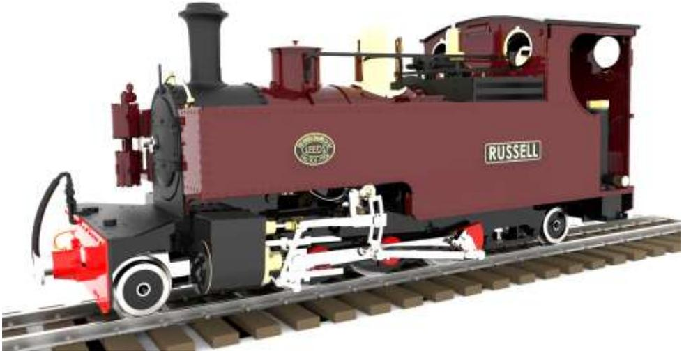
'Russell' is based on the well known 2-6-2 tank locomotive still running today on the Welsh Highland Railway in North Wales. Built by The Hunslet Engine Co. Ltd. of Leeds in 1906, it has undergone a number of changes over the years and the model depicts it as running in the early 1920's and as it currently appears.
