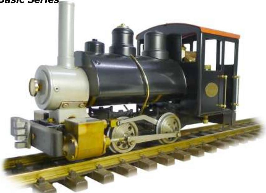
'Sammie' is the second locomotive in our 'basic Series'. Offered in a ready to run form as illustrated above, this simple, slip-eccentric, internally gas fired model can be easily enhanced using our accessory packs.
